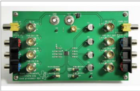
THS7372PWEVM, the THS7372 Evaluation Module, Top View
